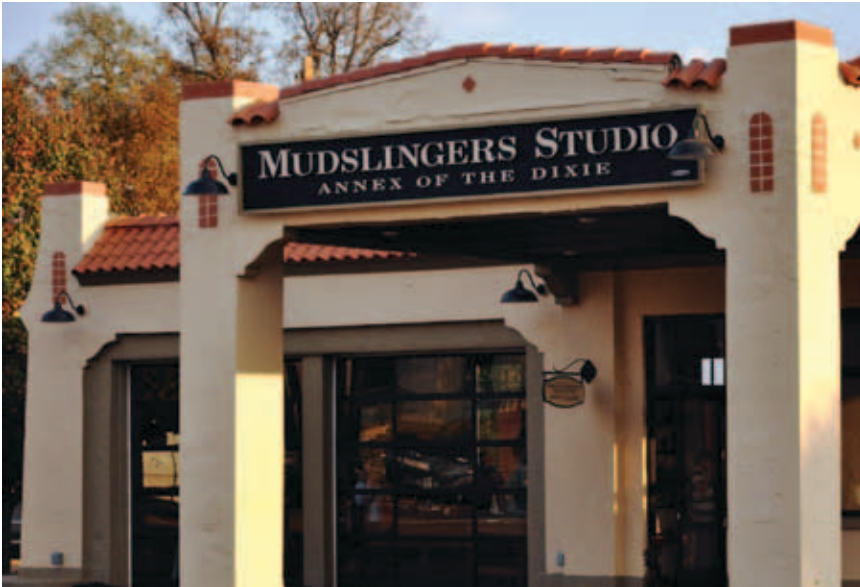
26-by-192-in. aluminum composite panel framed with aluminum box tubing, CNC-routed PVC letters over a Black Beauty sandblast slag background
