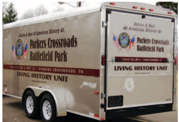
16-ft. cargo trailer lettered with computer-cut cast vinyl film and a digital print of the logo
