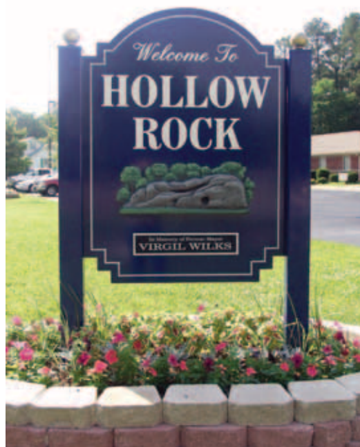
48-by-60-in. aluminum composite panel on PVC posts. The hand-carved HDU artwork represents the rock formation for which the town was named. Cast plaque by Grandview Aluminum.
