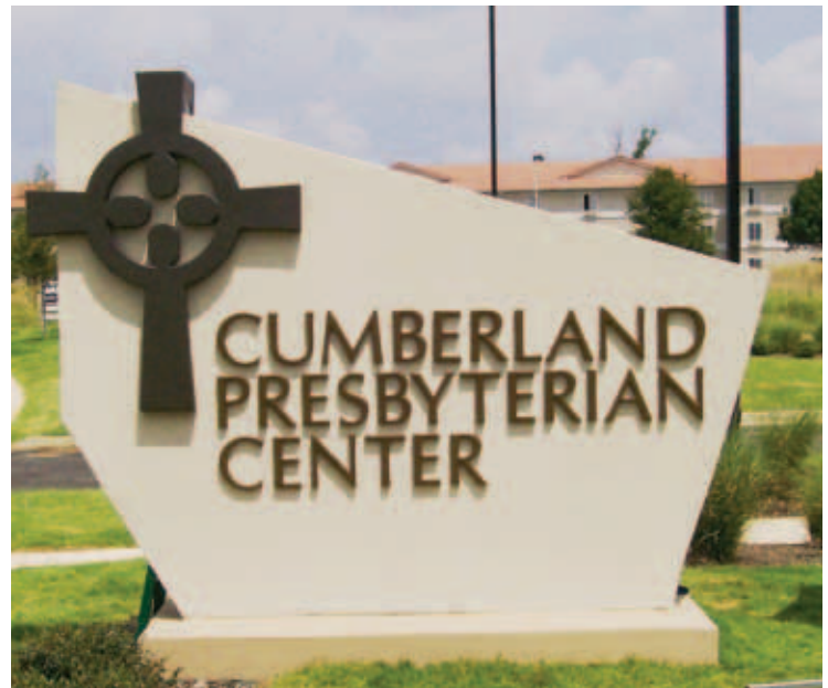
Monument for double-faced sign provided by builder; 8-in. formed Gemini letters with logo is cut from 2-in. EPS foam and coated with Chem-Coat 2538 two-part urethane, mounted on monument sign provided by builder. The acrylic latex finished logo wraps over the top and around the front edge of the 12-in.-thick sign structure.
