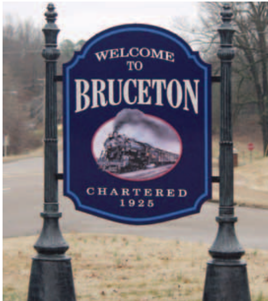
48-by-62-in. aluminum composite panel with cast vinyl film letters and a digital print
