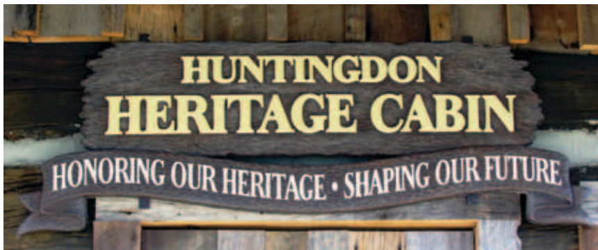
18-by-48-in. HDU panel finished in acrylic latex paint. The "weathered plank" effect leaves the primary lettering raised.
