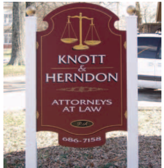
36-by-50-in. double-faced panel built from three panels of 1/2-in. overlaid plywood; enamel paint finish with a hand-painted pictorial and vinyl film graphics
