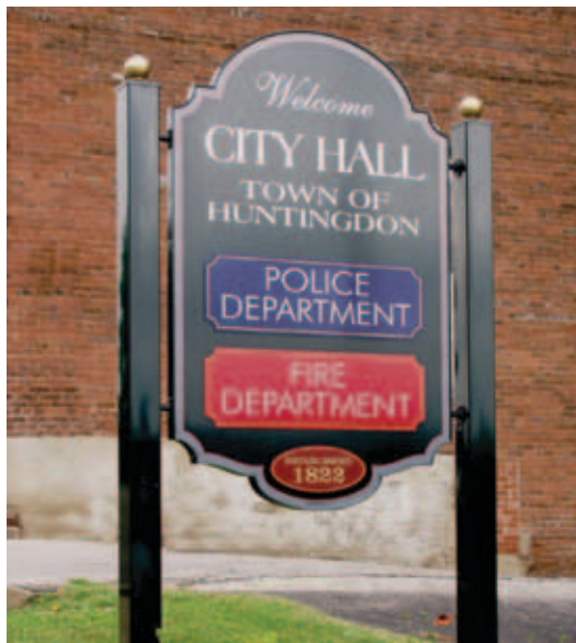
48-by-60-in. double-faced sign in a wooden frame, skinned and edge-wrapped with Alucobond aluminum composite material, mounted on PVC posts, sign face painted with lettering enamels, vinyl graphics
